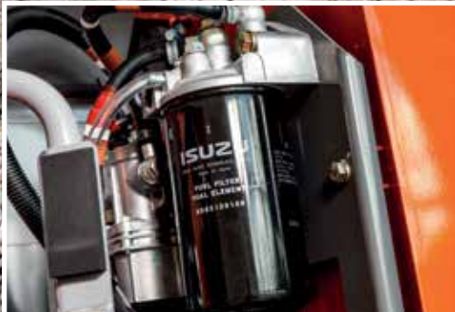
The main fuel filter is easier to replace.
